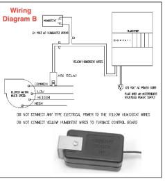
11b. Wiring Diagram B: Multi-Speed Blower. For wiring with a multi-speed blower, use an HUM-A50 Current Sensing Relay with an existing or independently wired, field-installed 120 VAC outlet. Plug the humidifier into the outlet.
